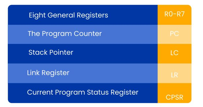
In thumb state, the higher registers (r8-r12) are not part of the standard register set.
